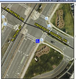
N TRYON ST Street 1 Name Stop Condition-Street 2 Signal Street 2 Name N/A Stop Condition-Street 1 N/A Possible Solutions: Remove & Replace Entire Ramp. Remove & Replace Gutter. Surveyor Notes: N/A PROW/ADA: R304.5.3, R302.7.2
