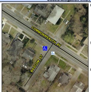
**BASCOM ST** Street 1 Name Stop Condition-Street 1 StopSign Street 2 Name N/A Stop Condition-Street 2 N/A Possible Solutions: Remove & Replace Entire Ramp. Surveyor Notes: N/A PROW/ADA: R304.5.1
