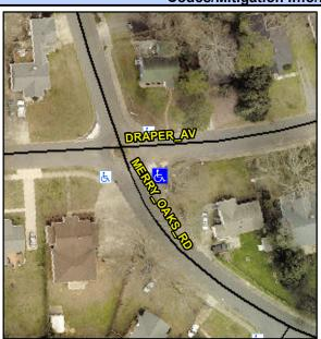
Street 1 Name Stop Condition-Street 2 Street 2 Name Stop Condition-Street 1 **DRAPER AV** YieldSign Remove & Replace Curb Ramp With Two New Directional Ramps or Equivalent.
