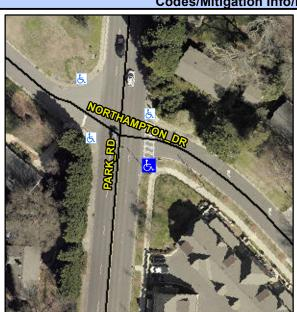
NORTHAMPTON DR Street 1 Name Stop Condition-Street 2 StopSign **PARK RD** Street 2 Name Stop Condition-Street 1 None Remove & Replace Curb Ramp With Two New Directional Ramps or Equivalent.
