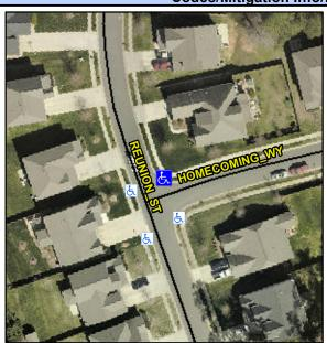
**REUNION ST** Street 1 Name Stop Condition-Street 2 None **HOMECOMING WY** Street 2 Name Stop Condition-Street 1 StopSign Possible Solutions: Remove & Replace Curb Ramp With Two New Directional Ramps or Equivalent. Surveyor Notes: N/A PROW/ADA:
