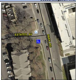
Street 1 Name **PARK RD** Stop Condition-Street 2 None **ESTATES AV** Street 2 Name Stop Condition-Street 1 StopSign Possible Solutions: Compliance Description N/A Remove & Replace Curb Ramp With Two New Directional Ramps or Equivalent. Surveyor Notes: N/A PROW/ADA: Not Found, R304.5.1, R304.2.2
