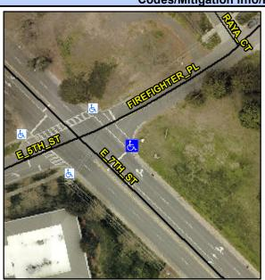
FIREFIGHTER PL Street 1 Name Stop Condition-Street 2 Signal Street 2 Name E 7TH ST Stop Condition-Street 1 Signal Possible Solutions: Remove & Replace Curb Ramp With **Two New Directional Ramps or** Equivalent. Surveyor Notes: N/A PROW/ADA: Not Found, R304.2.2
