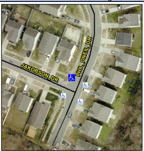
Street 1 Name Stop Condition-Street 1 Street 2 Name Stop Condition-Street 2 **JAKOBSON DR** StopSign **PHIL ONEIL DR** None Possible Solutions: Remove & Replace Curb Ramp With Two New Directional Ramps or Equivalent. Surveyor Notes: N/A PROW/ADA: Not Found, R304.5.1, R304.5.3
