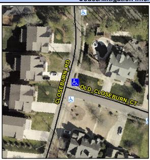
**CLOSEBURN RD** Street 1 Name Stop Condition-Street 2 **OLD CLOSEBURN CT** Street 2 Name Stop Condition-Street 1 StopSign Possible Solutions: Remove & Replace Curb Ramp With Two New Directional Ramps or Equivalent. Surveyor Notes: N/A PROW/ADA: R304.5.1
