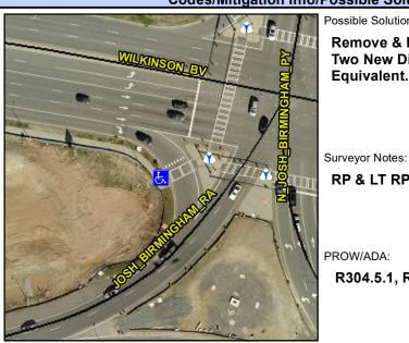
**WILKINSON BV** Street 1 Name Stop Condition-Street 1 YieldSign Street 2 Name N/A Stop Condition-Street 2 N/A Possible Solutions: Remove & Replace Curb Ramp With **Two New Directional Ramps or** Equivalent.
