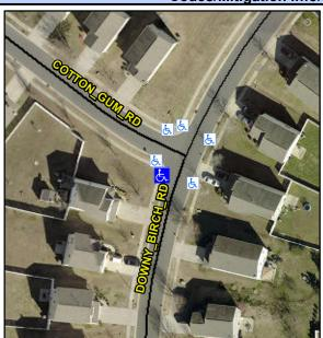
DOWNY BIRCH RD Street 1 Name Stop Condition-Street 1 None N/A Street 2 Name Stop Condition-Street 2 N/A Possible Solutions: Compliance Description Remove & Replace Curb Ramp With Two New Directional Ramps or Equivalent. Surveyor Notes: N/A PROW/ADA: Not Found, R304.5.3
