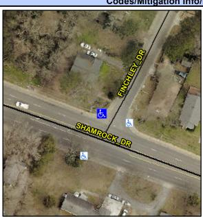
Street 1 Name Stop Condition-Street 2 Street 2 Name Stop Condition-Street 1 SHAMROCK DR None **FINCHLEY DR** StopSign Possible Solutions: Remove & Replace Curb Ramp With Two New Directional Ramps or Equivalent.
