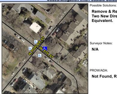
Street 1 Name Stop Condition-S Street 2 Name Stop Condition-S Remove & Replace Curb Ramp With Two New Directional Ramps or Equivalent.
