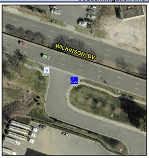
Wilkinson Street 1 Name Stop Condition-Street 2 None Street 2 Name **ENTRANCE** Stop Condition-Street 1 None Possible Solutions: Remove & Replace Curb Ramp With **Two New Directional Ramps or** Equivalent. Surveyor Notes: N/A PROW/ADA: Not Found, R304.2.2
