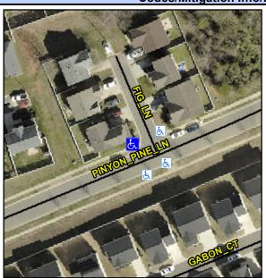
**PINYON PINE LN** Street 1 Name Stop Condition-Street 2 None FIG LN Street 2 Name Stop Condition-Street 1 StopSign Possible Solutions: Compliance Description N/A Remove & Replace Curb Ramp With Two New Directional Ramps or No Equivalent. Surveyor Notes: N/A PROW/ADA: Not Found, R304.5.1
