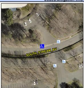
**SOUTHSTREAM BV** Street 1 Name Stop Condition-Street 2 None Street 2 Name **ENTRANCE** Stop Condition-Street 1 StopSign Remove & Replace Curb Ramp With Two New Directional Ramps or Equivalent.
