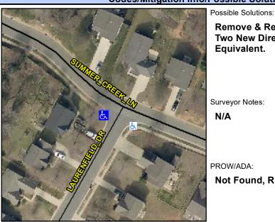
LAURENFIELD DR Street 1 Name Stop Condition-Street 1 StopSign Street 2 Name N/A Stop Condition-Street 2 N/A **Remove & Replace Curb Ramp With Two New Directional Ramps or** Equivalent.
