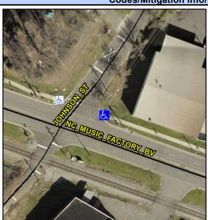
**JOHNSON ST** Street 1 Name Stop Condition-Street 1 StopSign Street 2 Name N/A Stop Condition-Street 2 N/A Possible Solutions: Remove & Replace Entire Ramp. Surveyor Notes: N/A R304.2.2, R304.5.3
