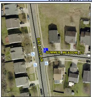
**DAY LILLY LN** Street 1 Name Stop Condition-Street 2 **SUMMER MEADOW CT** Street 2 Name Stop Condition-Street 1 StopSign Possible Solutions: Remove & Replace Curb Ramp With Two New Directional Ramps or Equivalent. Surveyor Notes: N/A PROW/ADA: R304.5.1, R304.2.2, R304.5.3
