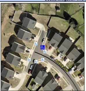
**AGAVA LN** Street 1 Name Stop Condition-Street 1 None Street 2 Name N/A Stop Condition-Street 2 N/A Possible Solutions: Remove & Replace Curb Ramp With Two New Directional Ramps or Equivalent. Surveyor Notes: N/A PROW/ADA: Not Found, R304.5.3
