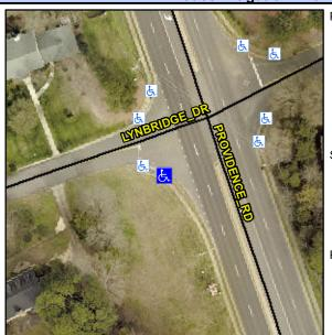
**PROVIDENCE RD** Street 1 Name Stop Condition-Street 2 None Street 2 Name N/A Stop Condition-Street 1 N/A Possible Solutions: Remove & Replace Entire Ramp. Surveyor Notes: N/A PROW/ADA: R304.5.1, R304.2.2
