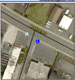
Street 1 Name Stop Condition-Street 2 Street 2 Name Stop Condition-Street 1 MONROE RD None **BUFORD AV** StopSign Possible Solutions: Remove & Replace Curb Ramp With **Two New Directional Ramps or** Equivalent. Surveyor Notes: N/A PROW/ADA: Not Found, R304.5.1, R304.2.2
