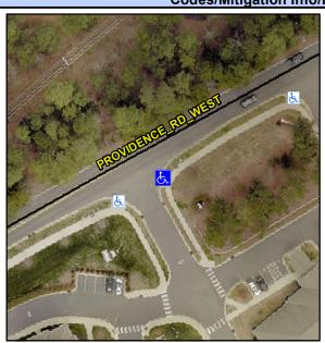
PROVIDENCE RD WEST Street 1 Name Stop Condition-Street 2 None **ENTRANCE** Street 2 Name Stop Condition-Street 1 StopSign Possible Solutions: Remove & Replace Curb Ramp With Two New Directional Ramps or Equivalent. Surveyor Notes: N/A PROW/ADA: R304.2.2
