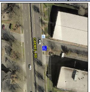
**ENTRANCE** Street 1 Name Stop Condition-Street 2 None **CARMEL RD** Street 2 Name Stop Condition-Street 1 None Possible Solutions: Compliance Description N/A Remove & Replace Curb Ramp With Two New Directional Ramps or Yes Equivalent. N/A N/A N/A N/A Surveyor Notes: N/A N/A N/A N/A N/A N/A PROW/ADA N/A Not Found, R304.5.3 N/A N/A N/A N/A
