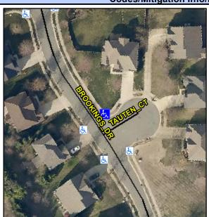
Street 1 Name Stop Condition-Street 2 Street 2 Name Stop Condition-Street 1 **BROOKINGS DR** None **TAUTEN CT** StopSign Possible Solutions: Remove & Replace Curb Ramp With Two New Directional Ramps or Equivalent. Surveyor Notes: N/A PROW/ADA: R304.5.1
