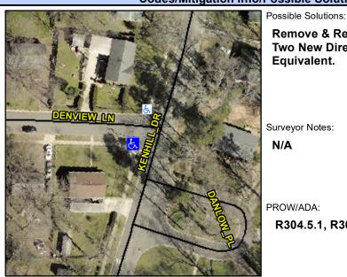
Stop Condition-Street 2 Street 2 Name Stop Condition-Street 1 **KENHILL DR** None **DENVIEW LN**  Remove & Replace Curb Ramp With Two New Directional Ramps or Equivalent.
