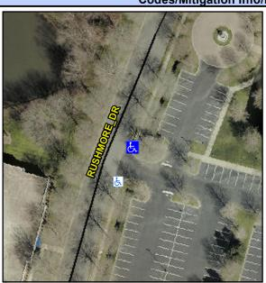
Street 1 Name Stop Condition-Street 2 Street 2 Name Stop Condition-Street 1 **RUSHMORE DR** None **ENTRANCE** StopSign Possible Solutions: Remove & Replace Curb Ramp With **Two New Directional Ramps or** Equivalent. Surveyor Notes: N/A PROW/ADA: Not Found, R304.5.1, R304.2.2, R304.5.3
