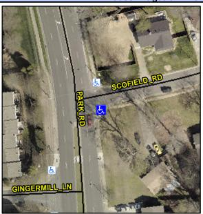
Street 1 Name **SCOFIELD RD** Stop Condition-Street 2 StopSign **PARK RD** Street 2 Name Stop Condition-Street 1 None Possible Solutions: Remove & Replace Curb Ramp With Two New Directional Ramps or Equivalent. Surveyor Notes: N/A PROW/ADA: Not Found, R304.2.2, R304.5.3
