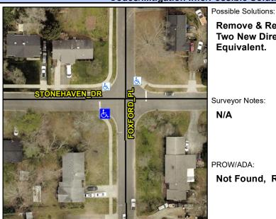
STONEHAVEN DR Street 1 Name Stop Condition-Street 1 StopSign Street 2 Name N/A Stop Condition-Street 2 N/A Remove & Replace Curb Ramp With Two New Directional Ramps or Equivalent.
