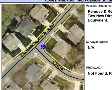
WEDGEWOOD COMMO Street 1 Name Stop Condition-Street 2 Street 2 Name MI Stop Condition-Street 1 Sto Remove & Replace Curb Ramp With **Two New Directional Ramps or** Equivalent.
