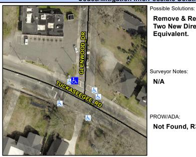
**GLENWOOD DR** Street 1 Name Stop Condition-Street 1 Signal Street 2 Name N/A Stop Condition-Street 2 N/A Remove & Replace Curb Ramp With Two New Directional Ramps or Equivalent.
