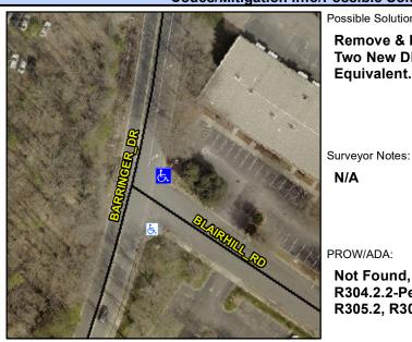
Street 1 Name Stop Condition-Street 2 Street 2 Name Stop Condition-Street 1 **BARRINGER DR** None **BLAIRHILL RD** StopSign Possible Solutions: Remove & Replace Curb Ramp With **Two New Directional Ramps or** Equivalent.
