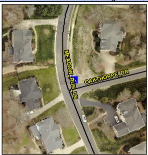
Street 1 Name Stop Condition-Street 2 Street 2 Name Stop Condition-Street 1 **MEADOW RUN LN** None **OAKTHORPE DR** StopSign Possible Solutions: Remove & Replace Curb Ramp With **Two New Directional Ramps or** Equivalent. Surveyor Notes: N/A PROW/ADA: R304.5.1, R304.5.3
