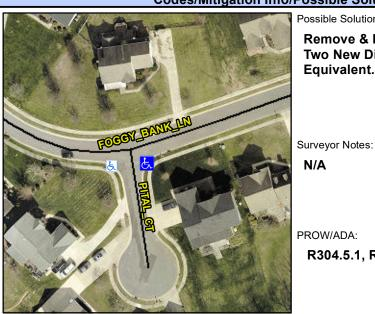
**PITAL CT** Street 1 Name Stop Condition-Street 1 StopSign Street 2 Name N/A Stop Condition-Street 2 N/A Possible Solutions: Remove & Replace Curb Ramp With **Two New Directional Ramps or** Equivalent.
