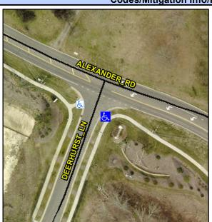
Street 1 Name Stop Condition-Street 1 Street 2 Name Stop Condition-Street 2 **ALEXANDER RD** None **DEERHURST LN** StopSign Possible Solutions: Remove & Replace Curb Ramp With Two New Directional Ramps or Equivalent. Surveyor Notes: N/A PROW/ADA: R304.5.1, R304.5.3
