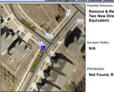
TREESDALE LN Street 1 Name Stop Condition-Street 1 None Street 2 Name N/A Stop Condition-Street 2 N/A **Remove & Replace Curb Ramp With Two New Directional Ramps or** Equivalent.
