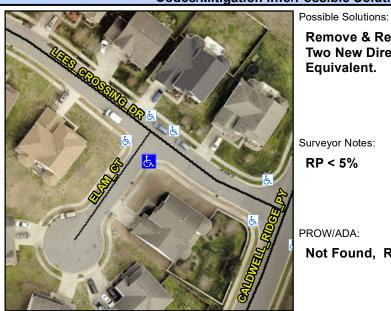
LEES CROSSING DR Street 1 Name Stop Condition-Street 1 Street 2 Name **ELAM CT** Stop Condition-Street 2 StopSign **Remove & Replace Curb Ramp With Two New Directional Ramps or** Equivalent.
