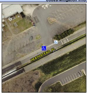
**HEATHSTEAD PL** Street 1 Name Stop Condition-Street 2 None **ENTRANCE** Street 2 Name Stop Condition-Street 1 None Possible Solutions: Remove & Replace Curb Ramp With Two New Directional Ramps or Equivalent. Surveyor Notes: N/A PROW/ADA: Not Found, R304.5.3
