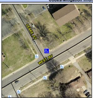
**LEAKE ST** Street 1 Name Stop Condition-Street 2 StopSign **WEST BV** Street 2 Name Stop Condition-Street 1 None Possible Solutions: Remove & Replace Curb Ramp With Two New Directional Ramps or Equivalent. Surveyor Notes: N/A
