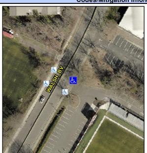
Street 1 Name Stop Condition-Street 2 Street 2 Name Stop Condition-Street 1 **WALSH BV** None **ENTRANCE** StopSign Possible Solutions: Remove & Replace Curb Ramp With **Two New Directional Ramps or** Equivalent. Surveyor Notes: N/A PROW/ADA: Not Found, R304.5.1, R304.2.2
