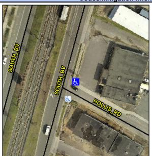
**SOUTH BV** Street 1 Name Stop Condition-Street 2 None Street 2 Name **HOLLIS RD** Stop Condition-Street 1 StopSign Possible Solutions: Remove & Replace Curb Ramp With Two New Directional Ramps or Equivalent. Surveyor Notes: N/A PROW/ADA: Not Found, R304.5.1, R304.2.2
