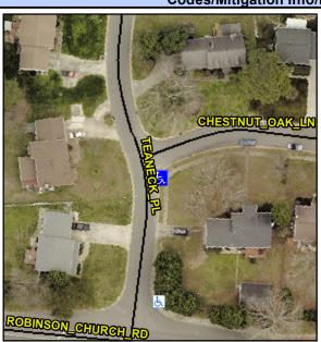
**CHESTNUT OAK LN** Street 1 Name Stop Condition-Street 2 StopSign **TEANECK PL** Street 2 Name Stop Condition-Street 1 None Possible Solutions: Remove & Replace Curb Ramp With Two New Directional Ramps or Equivalent. Surveyor Notes: N/A PROW/ADA: Not Found, R304.2.2
