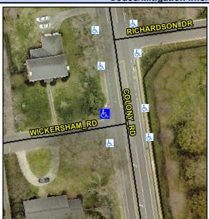
Street 1 Name Stop Condition-Street 2 Street 2 Name Stop Condition-Street 1 **WICKERSHAM RD** StopSign **COLONY RD** None Possible Solutions: Remove & Replace Curb Ramp With **Two New Directional Ramps or** Equivalent. Surveyor Notes: N/A PROW/ADA: R304.5.3
