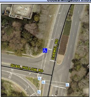
**QUAIL HOLLOW RD** Street 1 Name Stop Condition-Street 2 Signal **CARMEL RD** Street 2 Name Stop Condition-Street 1 Signal Possible Solutions: Remove & Replace Curb Ramp With **Two New Directional Ramps or** Equivalent. Surveyor Notes: N/A PROW/ADA: R304.2.2
