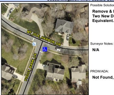
**FOGGY BANK LN** Street 1 Name StopSign Stop Condition-Street 1 Street 2 Name N/A Stop Condition-Street 2 N/A Possible Solutions: Remove & Replace Curb Ramp With Two New Directional Ramps or Equivalent.
