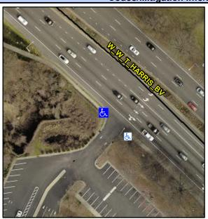
**ENTRANCE** Street 1 Name Stop Condition-Street 1 None Street 2 Name W W T HARRIS BV Stop Condition-Street 2 None Possible Solutions: Remove & Replace Curb Ramp With **Two New Directional Ramps or** Equivalent. Surveyor Notes: **MEDIAN ACROSS W W T HARRIS** BV PROW/ADA: R304.5.3, R304.3.2
