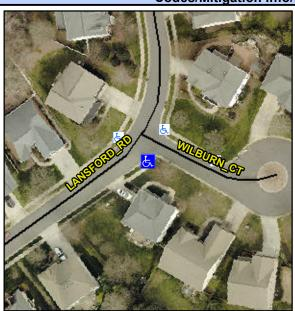
WILBURN CT Street 1 Name Stop Condition-Street 2 StopSign LANSFORD RD Street 2 Name Stop Condition-Street 1 None Possible Solutions: Remove & Replace Curb Ramp With Two New Directional Ramps or Equivalent. Surveyor Notes: N/A PROW/ADA: R304.5.3
