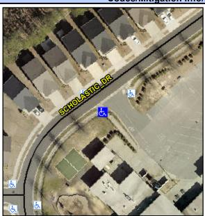
**ENTRANCE** Street 1 Name Stop Condition-Street 2 StopSign SCHOLASTIC DR Street 2 Name Stop Condition-Street 1 None Possible Solutions: Remove & Replace Curb Ramp With Two New Directional Ramps or Equivalent. Surveyor Notes: N/A PROW/ADA: R304.2.2
