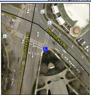
**PROVIDENCE RD** Street 1 Name Stop Condition-Street 2 Signal Street 2 Name **QUEENS RD** Stop Condition-Street 1 Signal Possible Solutions: Remove & Replace Curb Ramp With Two New Directional Ramps or **Equivalent. Restripe Crosswalk.** Surveyor Notes: N/A PROW/ADA: R304.5.1, R304.2.2, R304.5.3
