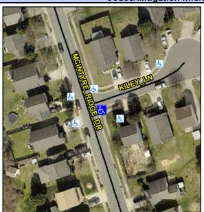
Street 1 Name StopSign Stop Condition-Street 1 KILEY LN Street 2 Name None Stop Condition-Street 2 MCINTYRE RIDGE DR Possible Solutions: Compliance Description N/A Remove & Replace Curb Ramp With Two New Directional Ramps or Yes Equivalent. Yes Yes N/A No Surveyor Notes: N/A RT RP < 5% N/A N/A N/A N/A PROW/ADA: N/A R304.5.1, R304.5.1, R304.5.3 N/A N/A N/A N/A N/A N/A
